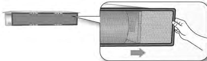
2. Clean the air filter with a vacuum or soft brush. If the dust is too thick, rinse them under running water and dry in a well-ventilated area.
