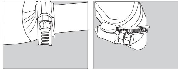
9. Install the drain pipe into the drain hose. Secure it with PVC adhesive and clamps as necessary to ensure a tight fit with no leakage.
