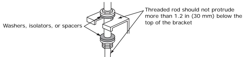
8. Maintain proper spacing between the unit and the ceiling; refer to the following figure.
