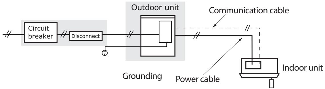
**Figure 2. Wiring terminals**
