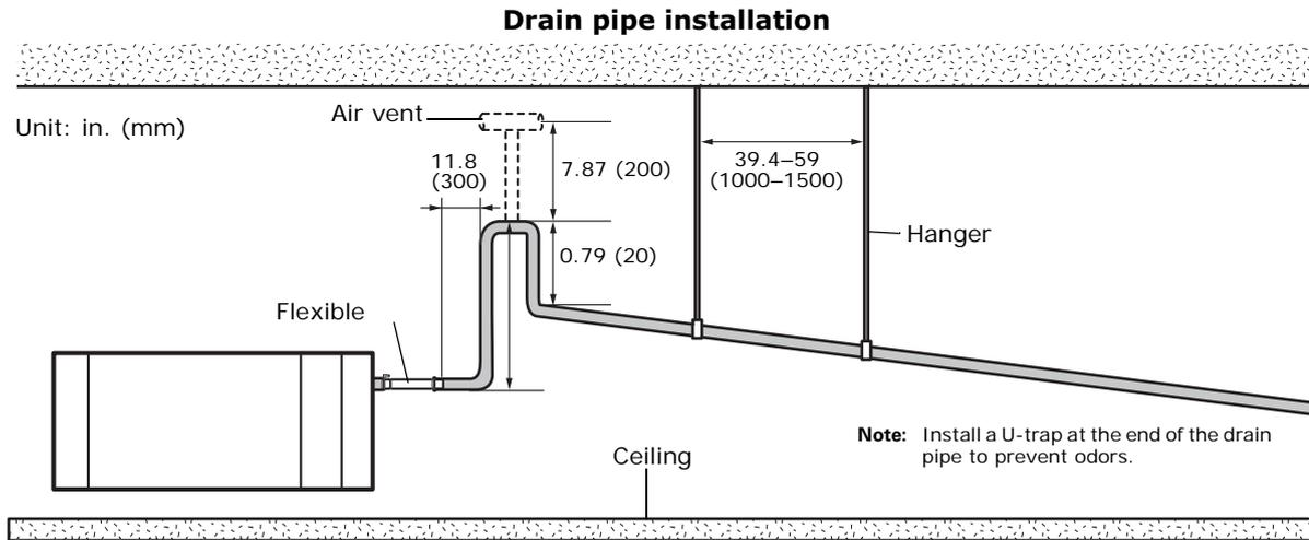
If the installation requires more than three indoor units, install the main air vent at the front of the indoor unit that is farthest from the main drain. It may be necessary to install individual air vents to prevent water flowing back to each indoor unit.
