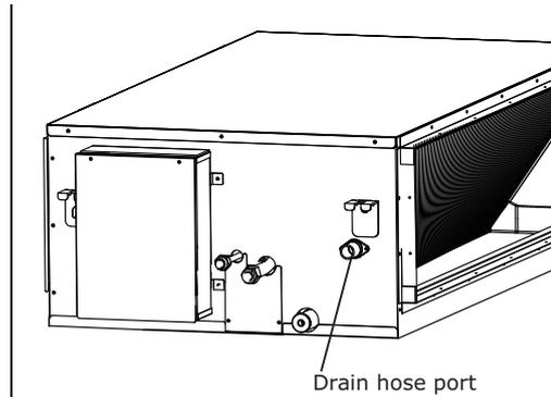
8. Wrap the insulation (supplied) around the drain hose and clamp the connection as tightly as possible until you can see at least 8 holes.
