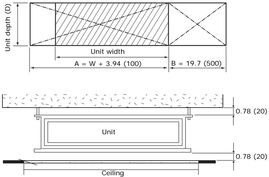
**Note:** If the unit is installed in a ceiling that does not have removable tiles, make allowances for servicing the unit by creating an access hole. If the unit is installed more than 39.4 in. (1 m) above the floor, the access hole must be the size of "B." If the unit is installed less than 39.4 in. (1 m) above the floor, the access hole must be the size of "A" + "B" both.
